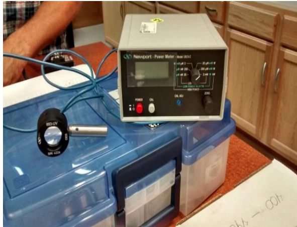
Figure 3. Equipment for measuring optical power of Laser Diode.
